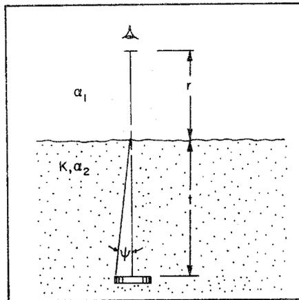
FIG. 1.55 Contrast reduction along a composite path through air, air-water surface, and water.
