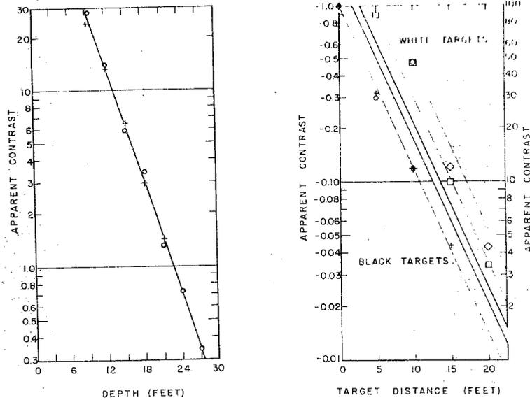
FIG. 1.29 Duntley's classic experiment showing the exponential law of decrease of apparent contrast along a vertical path in a natural hydrosol (Lake Winnepesaukee, N.H., Autumn, 1948. See also Figs. 1.28, 1.30)(Fig. 30, middle diagram, from [78], by permission)
