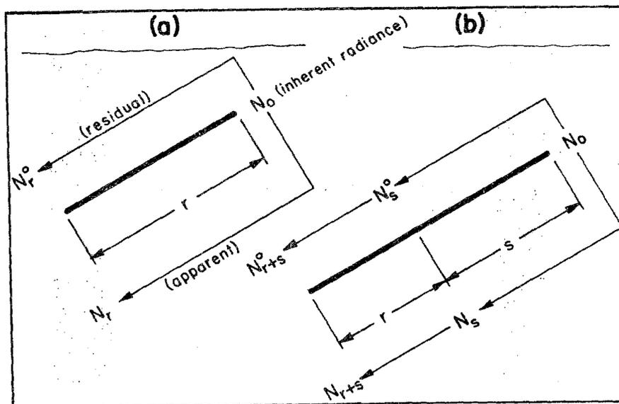
FIG. 1.54 Part (a): Deriving the contrast transmittance as the ratio of a residual radiance and an apparent radiance. Part (b): Deriving the multiplicative (or semigroup) property of contrast transmittance.
