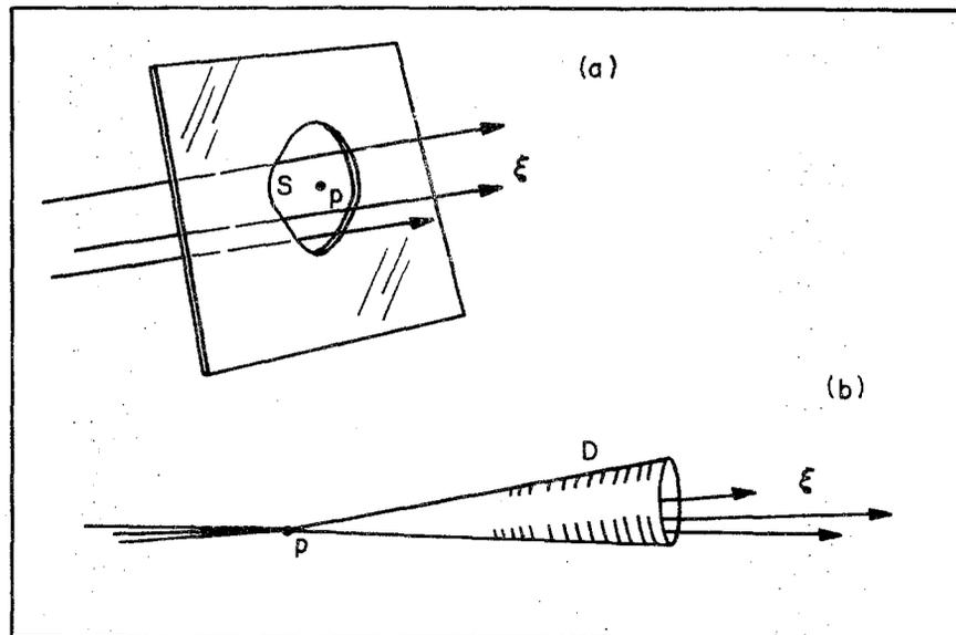
FIG. 1.4 Two geometric modes of describing radiant flux.
