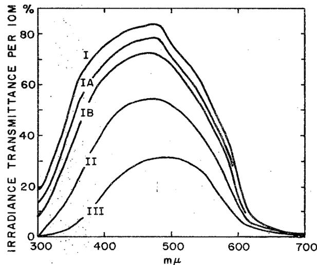
FIG. 1.74 Irradiance transmittance for a 10 meter layer of water, as sampled by Jerlov, and illustrating a possible classification scheme for natural hydrosols. (From [127], by permission)
