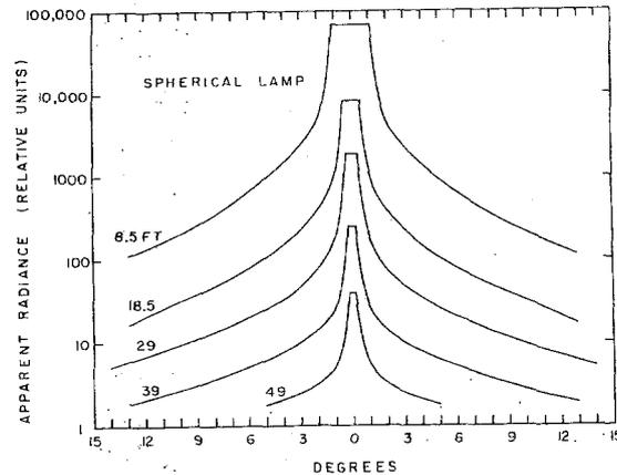
FIG. 1.61 Radiance distributions produced by a point source (small spherical lamp). Measured by Duntley, Lake Winnepesaukee, N.H., 3 August 1961. (Fig. 15 from [78], by permission)
