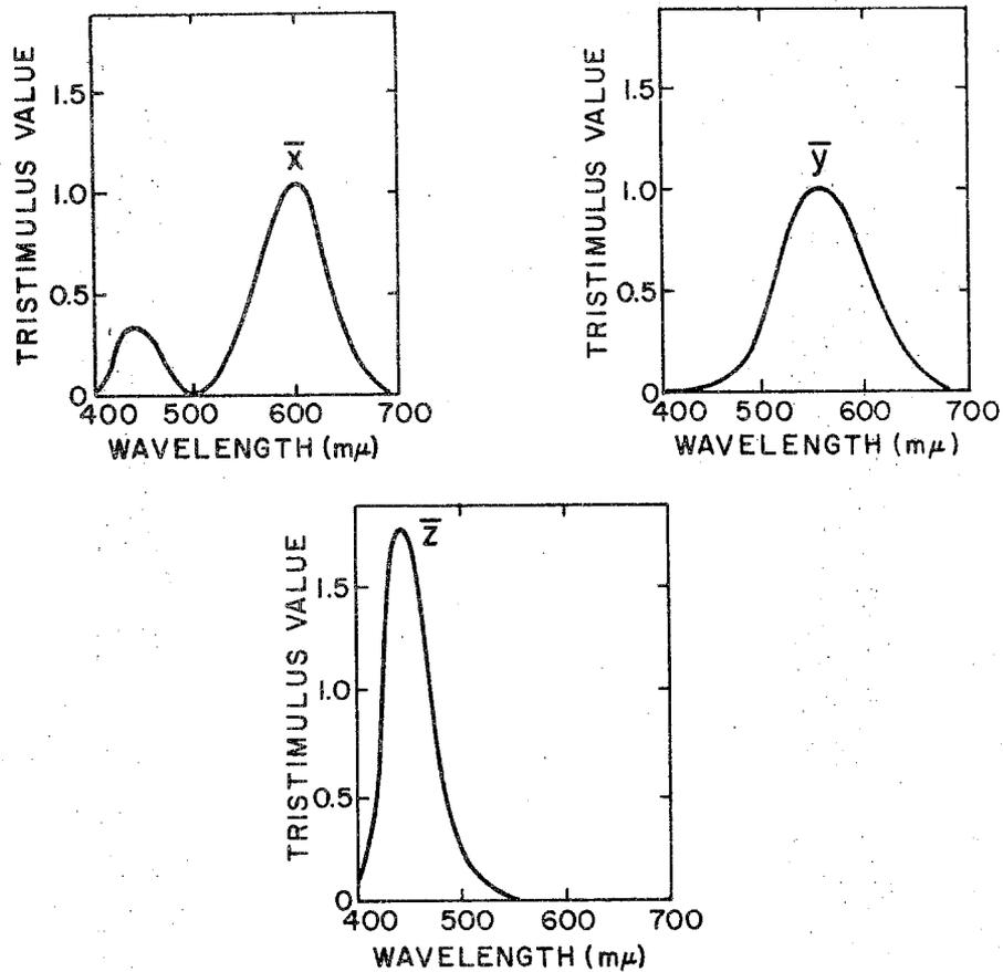
FIG. 1.76 The tristimulus functions. The  $\bar{y}$  curve is the photopic luminosity function of Fig. 1.10.
