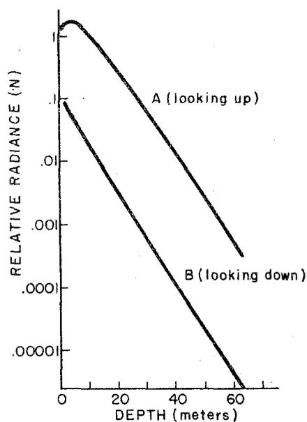
FIG. 1.22 Two experimental determinations of radiance by Tyler, Pend Oreille Lake, Idaho, April 1957. Note the general exponential decrease. Note, also, the slight buildup of radiance for the upward looking path near the surface. (From [298], by permission)
