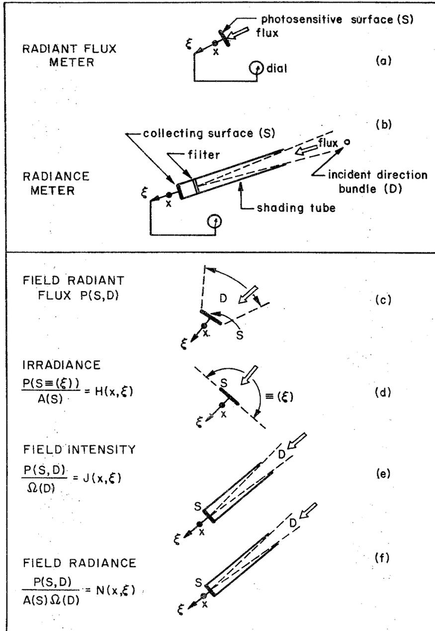
FIG. 1.5 Operational definitions of the radiometric concepts.
