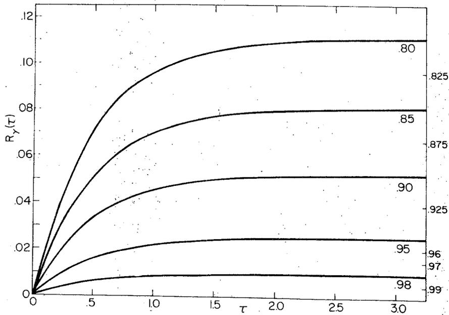
FIG. 1.41 Calculated reflectance  $R_Y(\tau)$  versus  $\tau$ , for  $.01 \leq \gamma \leq .80$ .
