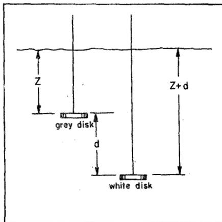
FIG. 1.56 The Duntley-disk procedure for measuring  $\alpha+K$ .
