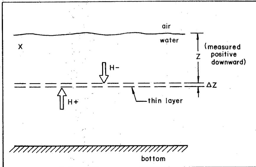
FIG. 1.38 Setting for the two-flow model for irradiance.
