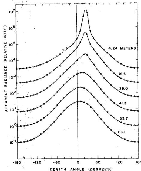
FIG. 1.23 Radiance distributions, in the vertical plane containing the sun, on a clear sunny day, at the indicated depth, in Lake Pend Oreille, Idaho, as measured by Tyler, April 1957. Observe how the shapes of the curves become similar as depth increases. (Fig. 26, from [78], by permission)
