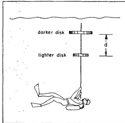
FIG. 1.57 The Duntley-disk procedure for measuring  $\alpha$ -K.
