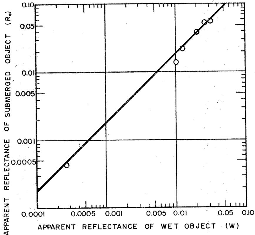
FIG. 1.87 Graphical means of determining the reflectance  $R_0$  of a submerged surface given its wet reflectance. The technique involves wetting the sample with a thin film of water, irradiating it with a beam at  $45^\circ$ , and viewing it normally, say with a conventional refractometer. This determines the abscissa of the graph. The associated ordinate yields  $R_0$ . This scheme was designed by Duntley, and the plotted points are the results of his experimental check of the graph.
