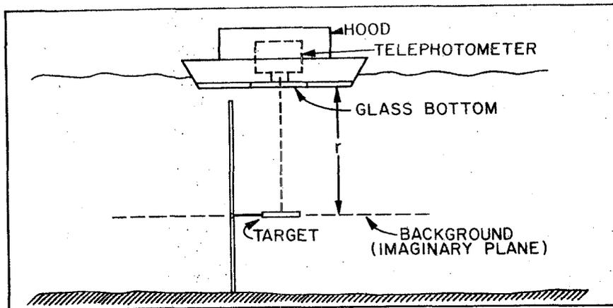
FIG. 1.28 Physical set-up for Figs. 1.29, 1.30.
