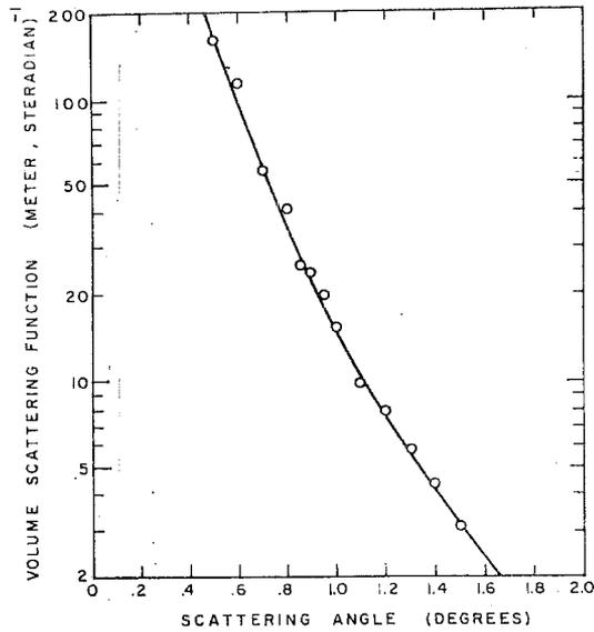
FIG. 1.72 Extreme detail of forward scattering values of volume scattering function in Duntley's lake water curve of Fig. 1.71.
