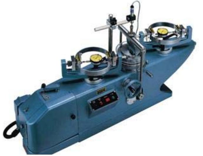
**Fig. 2:** Bromhead ring shear apparatus.
