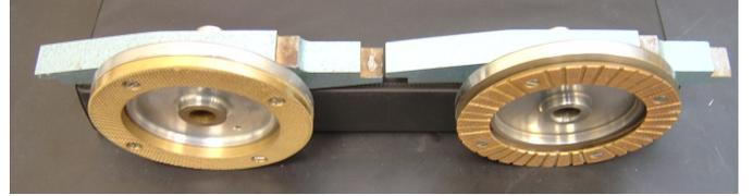
**Fig. 9:** Angle view that shows the difference between the original porous bronze platen (on the left) and the modified porous bronze platen (on the right).
