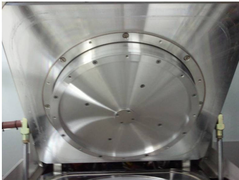
Figure 6.11 Top of the chamber with parts removed revealing the gas shower head. The gas enters through the center where it hits a baffle that redistributes the gas across the entire shower head area.
