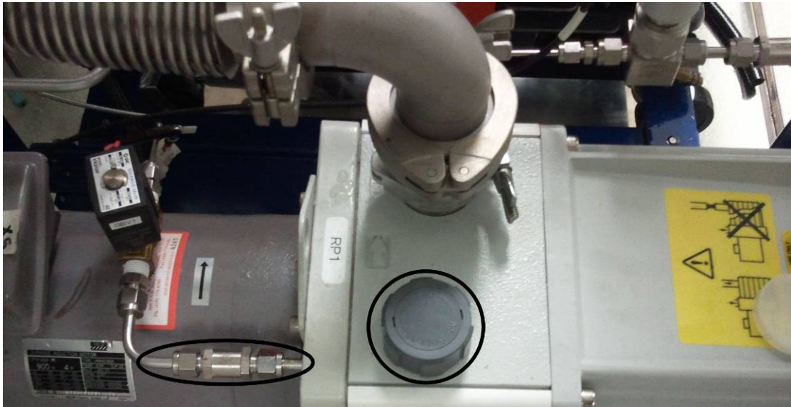
Figure 5.3 Top of E2M30 (RP1) showing the gas ballast inlet (left) and the ballast adjustment valve (right)
