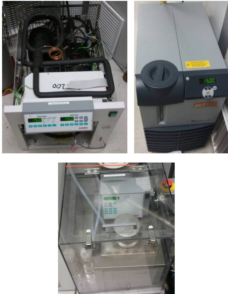
Figure 5.5 Left: Julabo FC1200- fluorine ICP chuck chiller, middle: ThermoFlex 1200- seal chiller for both ICPs, right: Julabo TD12- chuck heater for chlorine ICP
