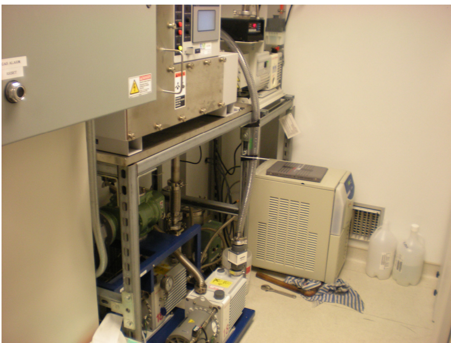
Figure 3.2 Top: Inside the PECVD chasing, viewed from the entrance, showing a gas cabinet on the left and two more on the back right. Bottom: The burn box, pumps and chiller located across from the back gas cabinets.
