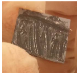
Figure 2.6 Sample with grease on the back of it. Notice how the grease covers the entire back of the sample. Because of this some, grease will come out from the sides when it is place on the carrier wafer but this also provides a uniform distribution under the sample.
