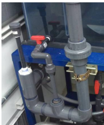
Figure 5.8 Side view of the scrubber. On the left is the red drain valve and on the right is the drain pipe that allows for continuous draining of water during operation.
