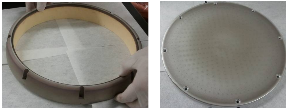
Figure 6.10 Top parts of the chamber. Left is the ground ring with the insulation ring installed inside it. Right is the shower head plate.
