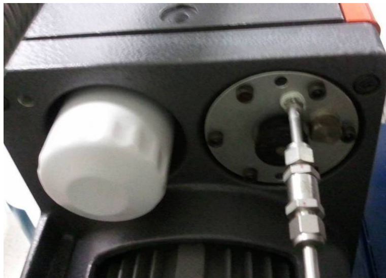
Figure 5.2 Back of the E2M40 showing the oil filter (left) and gas ballast inlet and valve (right)
