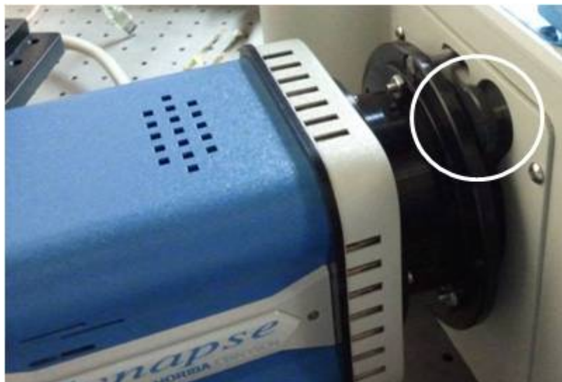
Figure 4.11 Mounting flange for connecting the CCD to the spectrometer. The circled item is a tilt adjustment screw.
