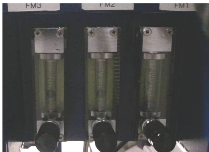
Figure 5.4 Gas ballast flow meters: Left to right these are the RP2 ballast, RP1 ballast, and Purge for RP1 (PV).
