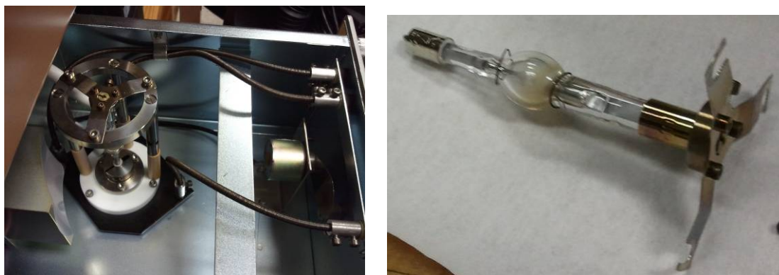
Figure 4.33 Left: the bulb in the assembly with the spring contacts on top. Right: the removed bulb with the spring contacts installed on the top of the bulb.
