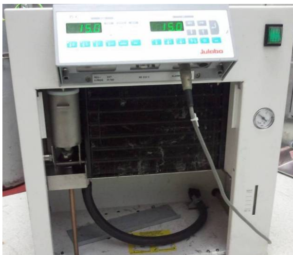
Figure 5.6 Front of the FC1200 chiller with front cover removed. From left to right: fill spout, interlock wire, drain hose and valve, and water level indicator.
