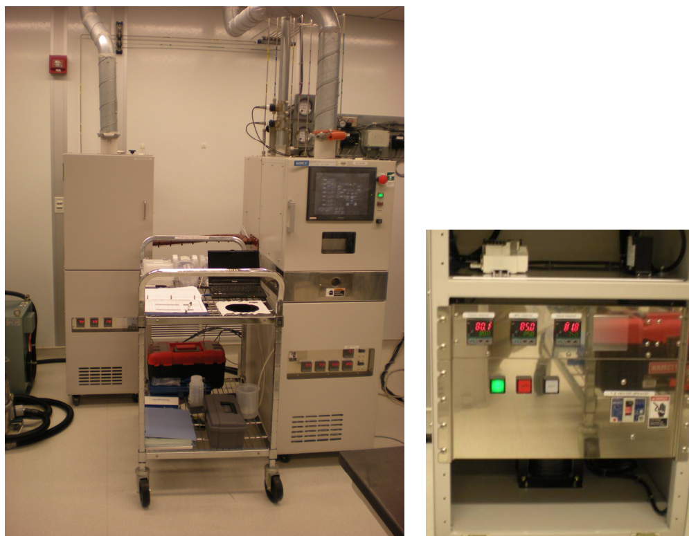
Figure 3.3 Left: The PECVD system with the TEOS cabinet on the left. Right: a close up of the heater controllers and on switch for the TEOS cabinet.
