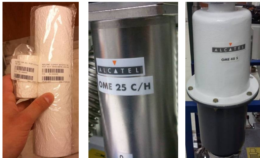
Figure 5.1 Left: Oil mist filters for the OME 25 C/H and OME 40 S respectively, Middle: OME 25 C/H, Right: OME 40 S
