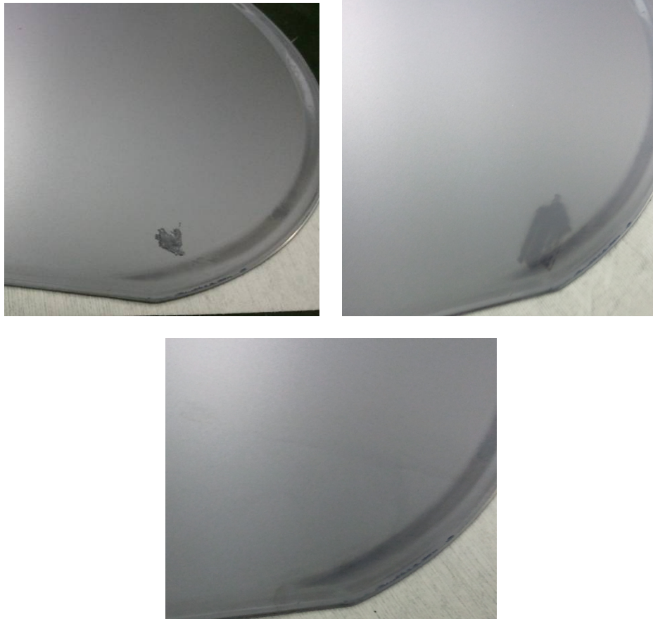
Figure 2.5 Top left: wafer with a large amount of vacuum grease on it. Top right: wafer with grease wiped off but residue still present. Bottom: wafer with the grease residue removed with IPA.
