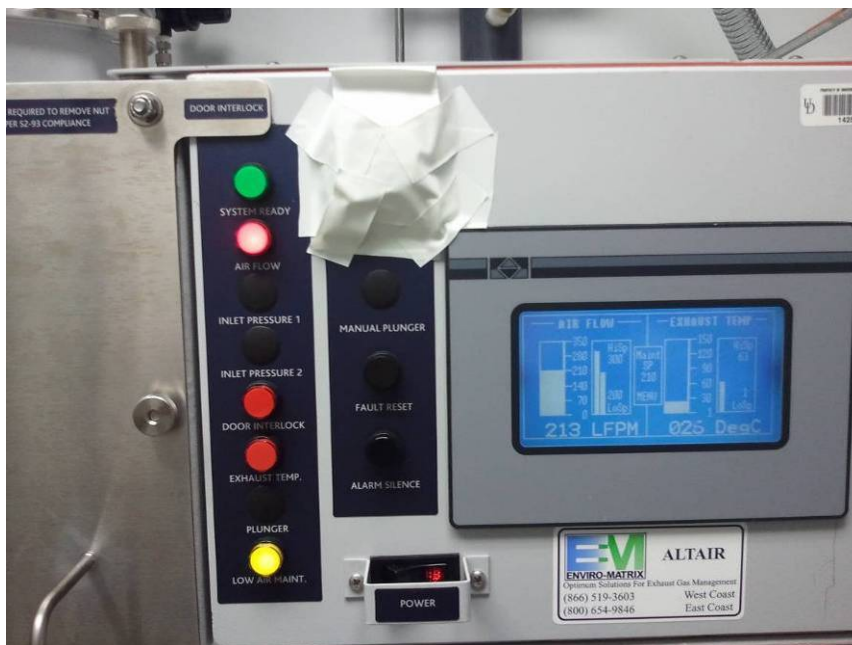
Figure 6.5 Front panel of the burn box showing the indicator lights, control switches, and display screen
