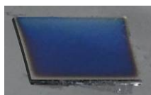
Figure 2.8 Silicon sample with oxide remaining after etch. This color oxide layer should be removed with approximately 1 minute of etching.
