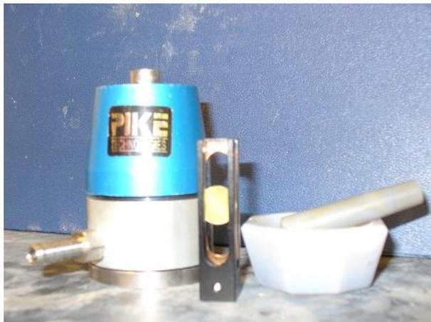
**Figure 15** The KBr pellet press, pellet clip, and mortar and pestle used to make pellets
