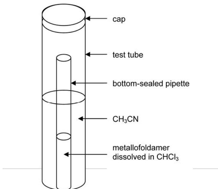
**Figure 14** Illustration of crystallization setup
