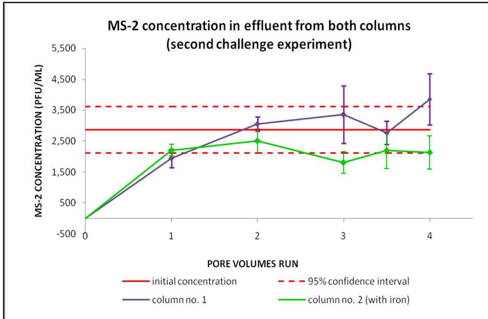
**Figure B.3 MS-2 removal in both columns on the 10<sup>th</sup> day of filters operation (preliminary experiment – samples analyzed one day after the experiment)**
