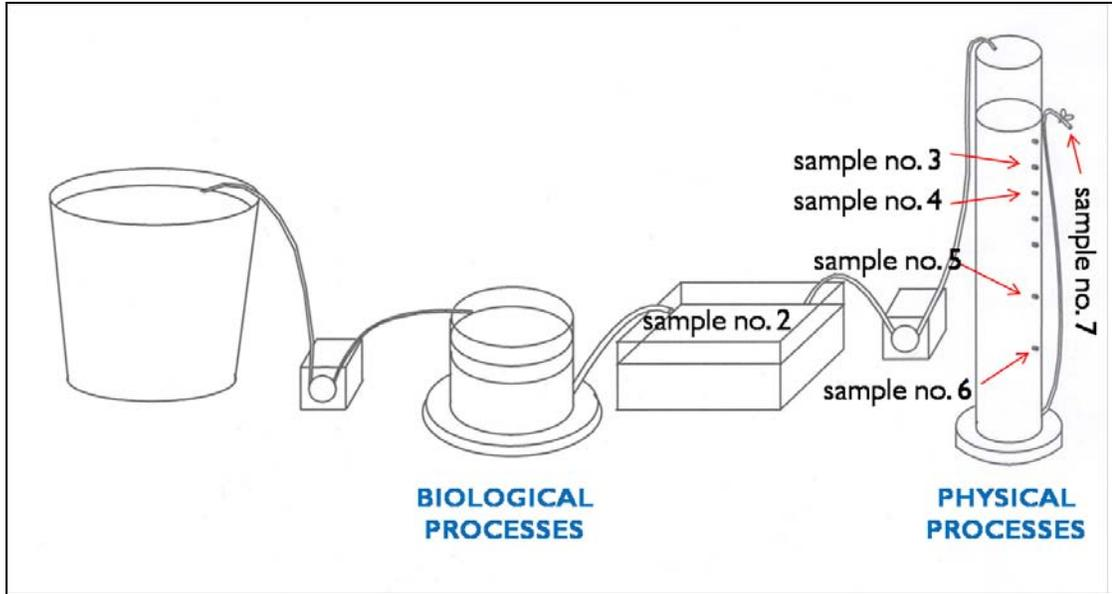
**Figure 3.1 Contribution of biological versus physical processes to pathogen removal in intermittent slow sand filtration (experimental setup).**
