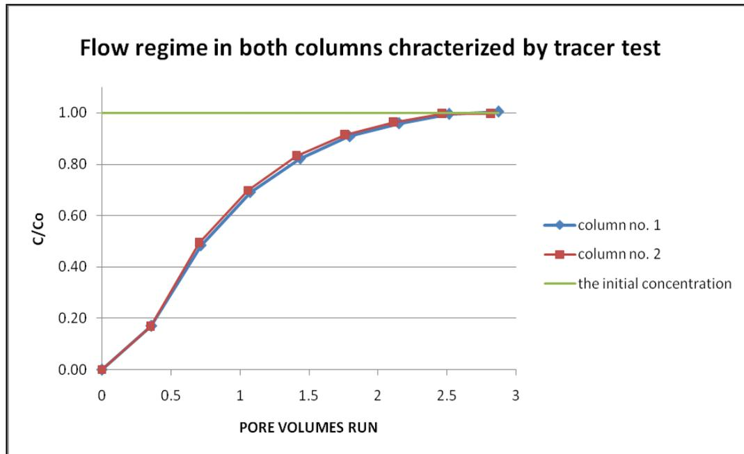
**Figure B.1** Flow regime in both columns characterized by tracer curves (preliminary experiment)
