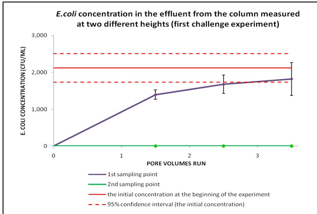
**Figure 4.8** *E. coli* removal by the schmutzdecke and by the ZVI layer on the 2<sup>nd</sup> day of filters operation
