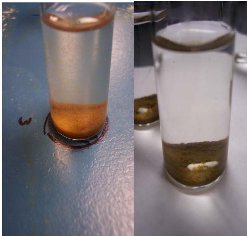
**Figure 3.2** Particles flocculating in the supernatant water poured out from the filter that was just cleaned
