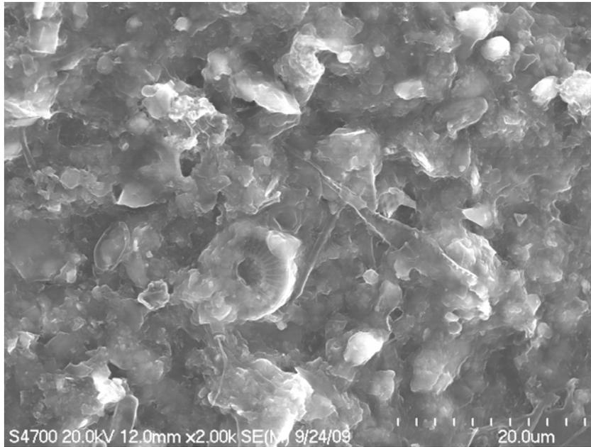
**Figure A.14 SEM picture of the schmutzdecke material (7)**
