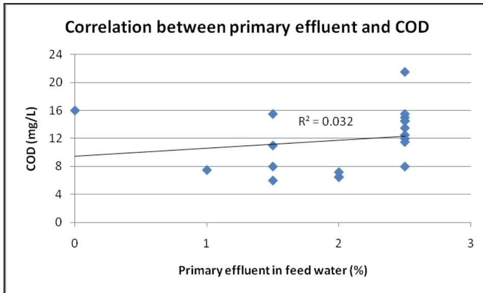
**Figure A.5** Correlation between primary effluent and the COD in the feed water
