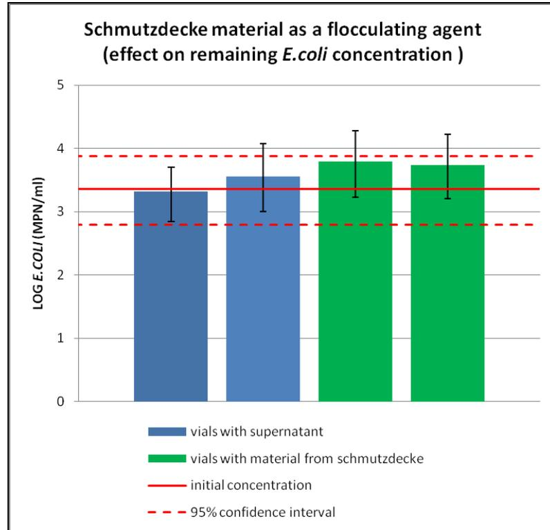
**Figure 3.15** The schmutzdecke material as a flocculating agent (effect on *E.coli* concentration)
