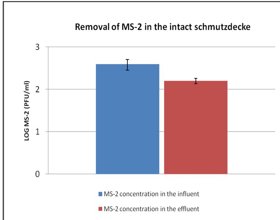
**Figure 3.12 Removal of MS-2 in the intact schmutzdecke**
