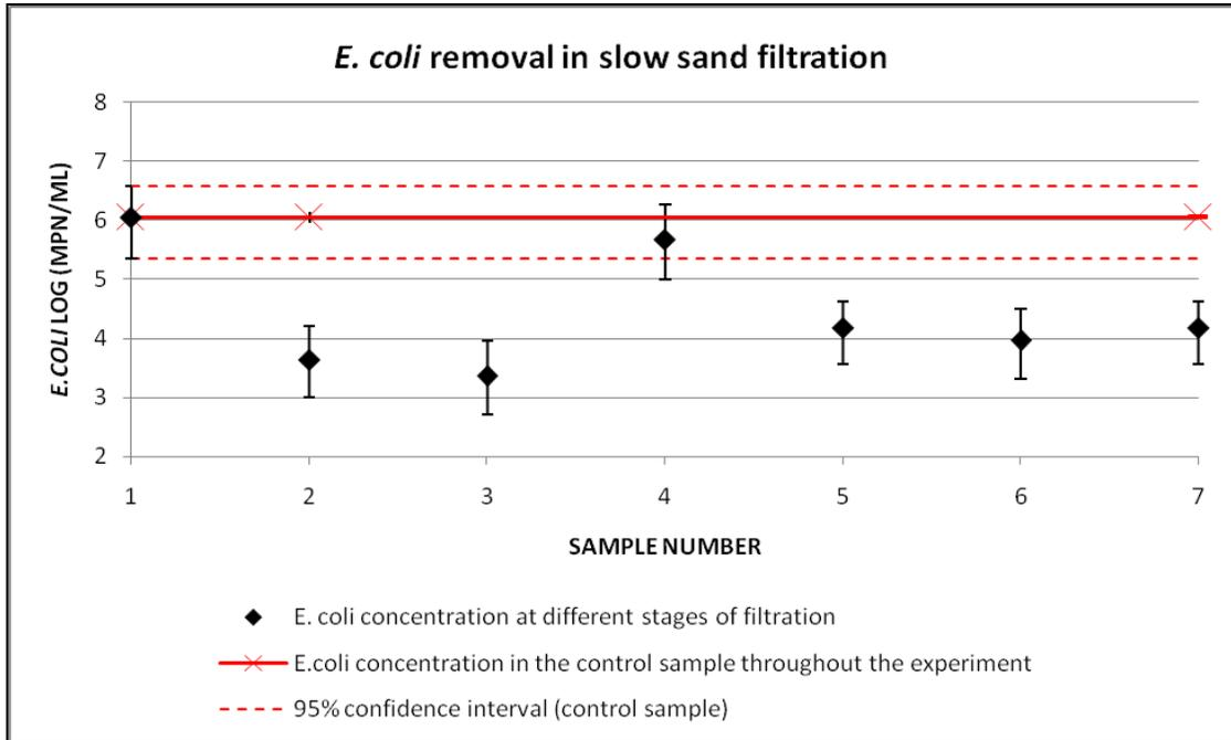
**Figure 3.4** *E.coli* removal due to biological versus physical processes in intermittent slow sand filtration
