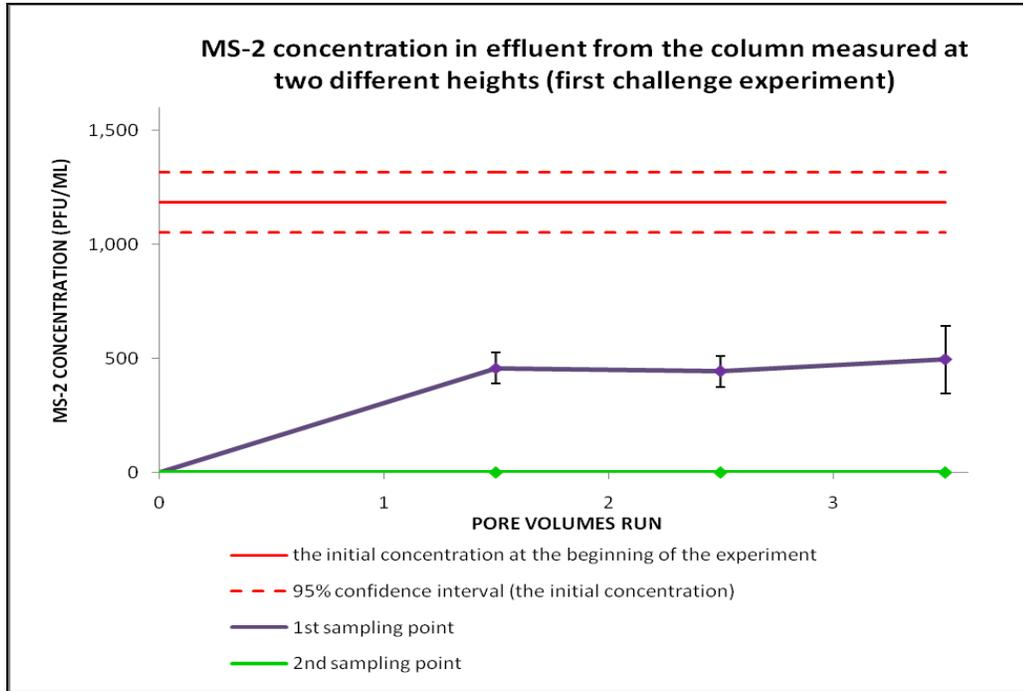
**Figure 4.9 MS-2 removal by the schmutzdecke and by the ZVI layer on the 2<sup>nd</sup> day of filters operation**
