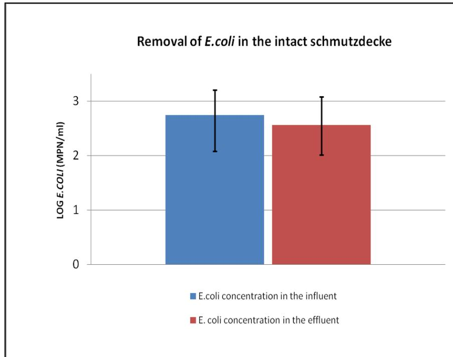
**Figure 3.10** Removal of *E.coli* in the intact schmutzdecke
