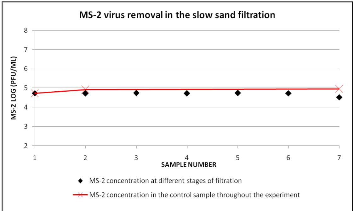
**Figure 3.5 MS-2 removal due to biological versus physical processes in intermittent slow sand filtration**
