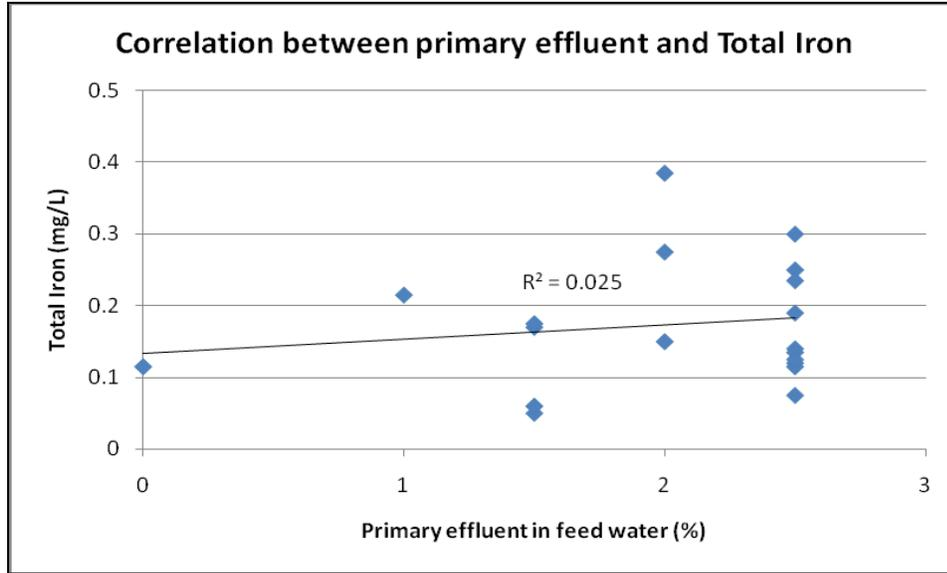
**Figure A.2 Correlation between primary effluent content and the total iron concentration in the feed water**
