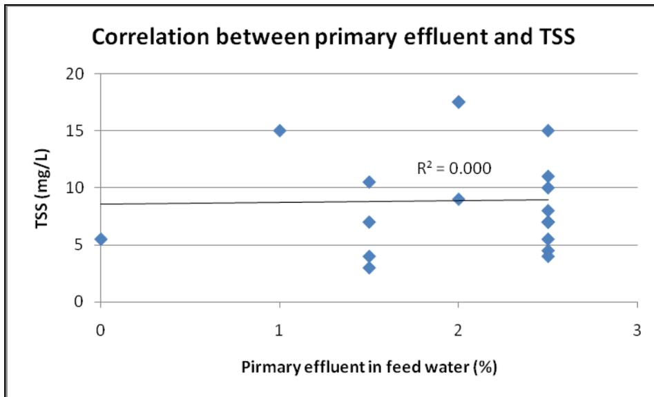
**Figure A.3 Correlation between primary effluent content and the TSS in the feed water**
