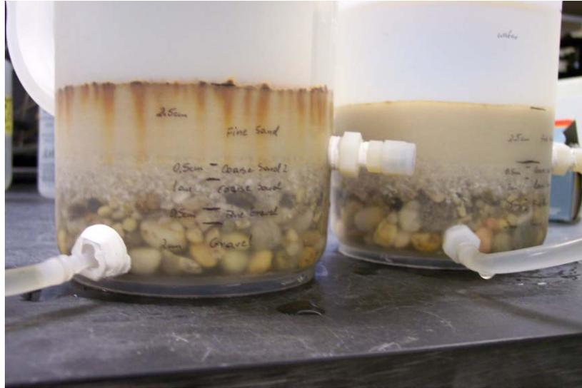
**Figure B.4** Uneven ripening of sand below the iron filings – 1
