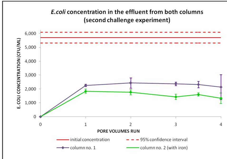
**Figure 4.5** *E. coli* removal in both columns on the 10<sup>th</sup> day of filters operation (preliminary experiment)
