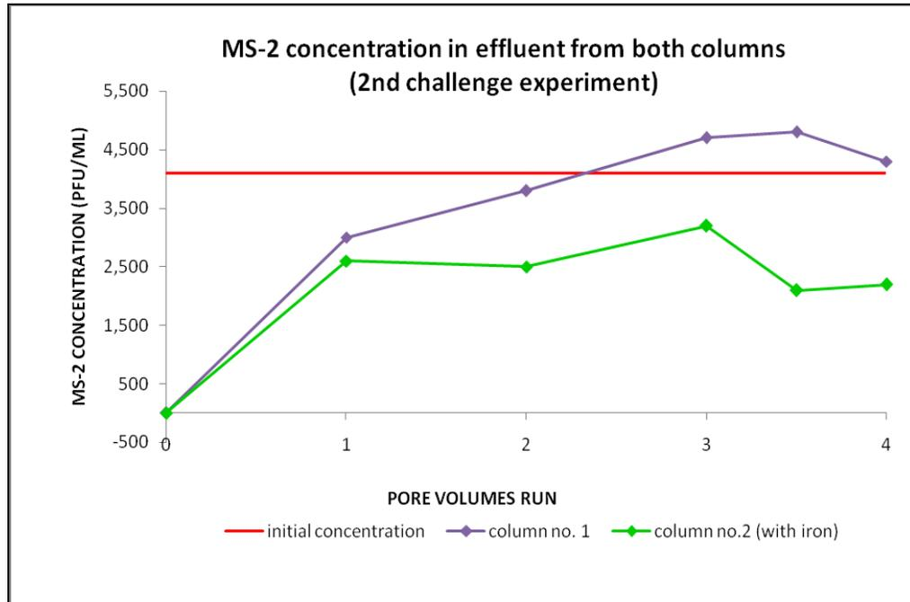
**Figure 4.7 MS-2 removal in both columns on the 10<sup>th</sup> day of filters operation (preliminary experiment)**
