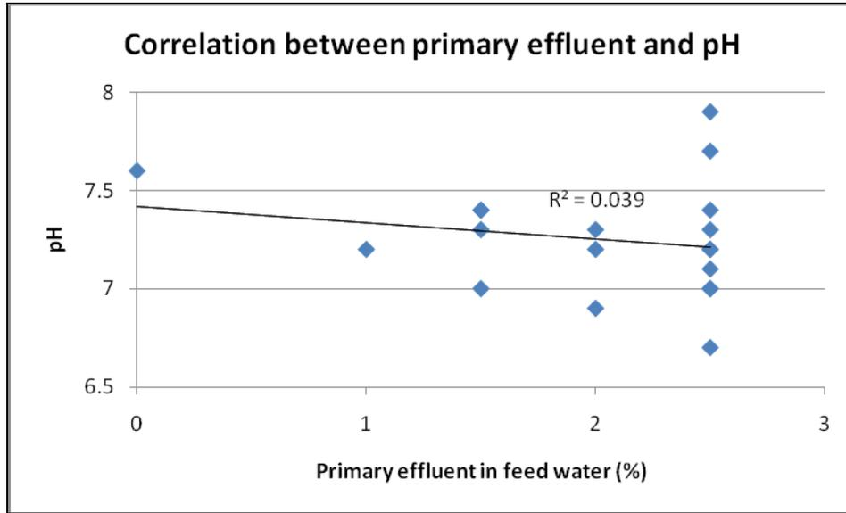
**Figure A.4** Correlation between primary effluent content and the pH in the feed water
