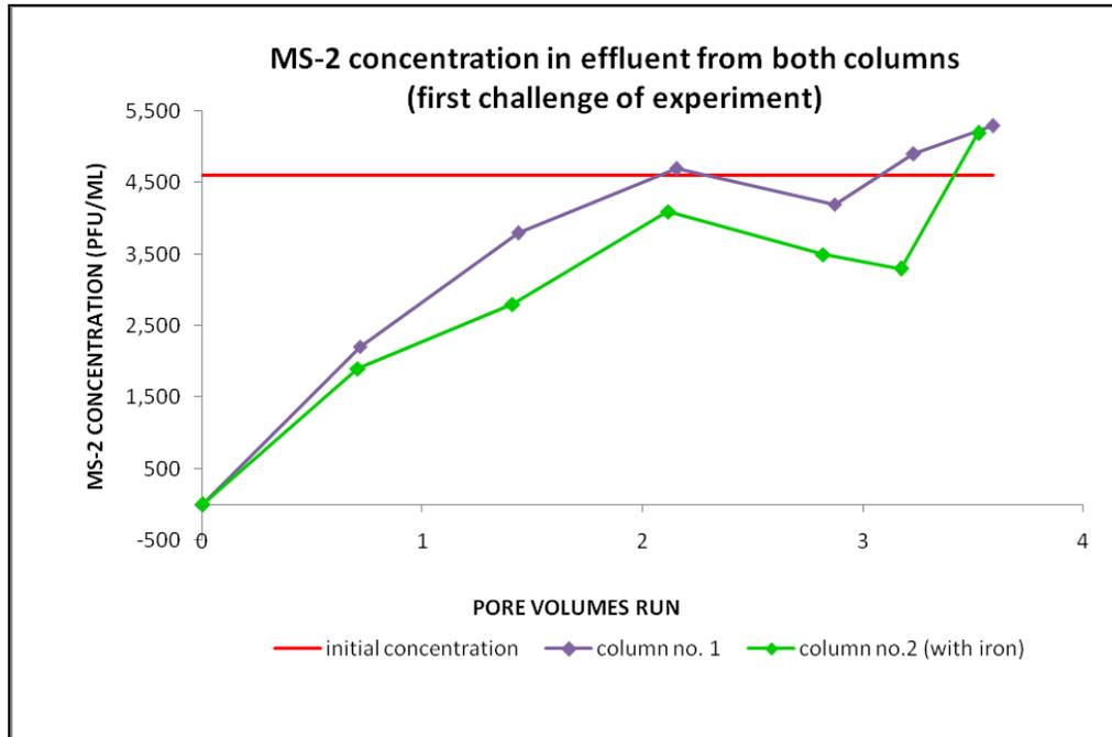
**Figure 4.6 MS-2 removal in both columns on the 2<sup>nd</sup> day of filters operation (preliminary experiment)**
