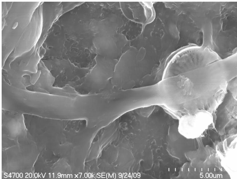
**Figure A.15 SEM picture of the schmutzdecke material (8)**
