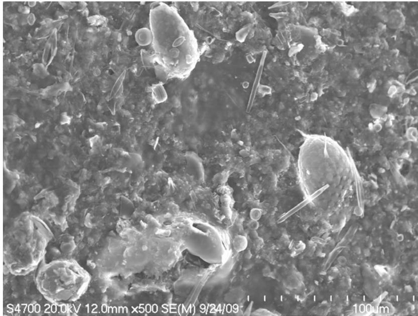
**Figure A.10 SEM picture of the schmutzdecke material (3)**
