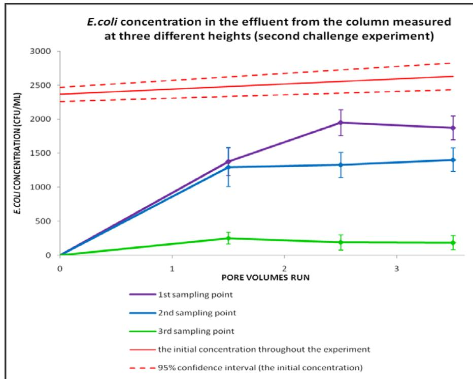
**Figure 4.10** *E. coli* removal by the schmutzdecke, by the sand underneath the schmutzdecke, and by the ZVI layer on the 19<sup>th</sup> day of filters operation
