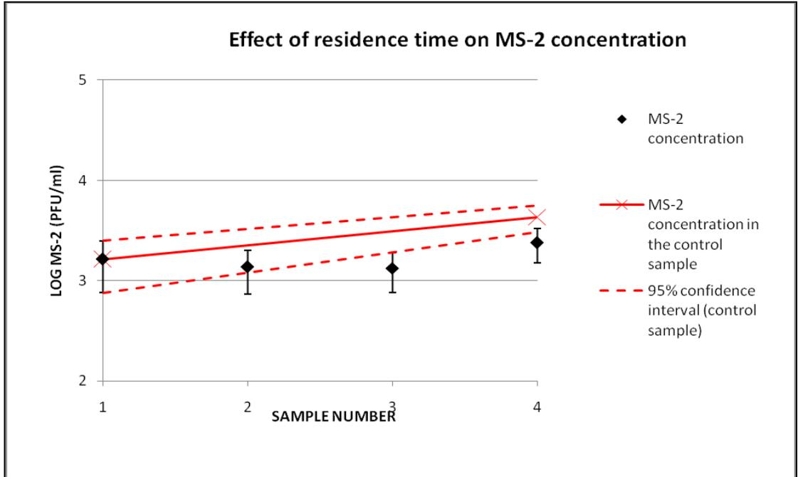
**Figure 3.7 Effect of residence time on MS-2 removal (first experiment)**
