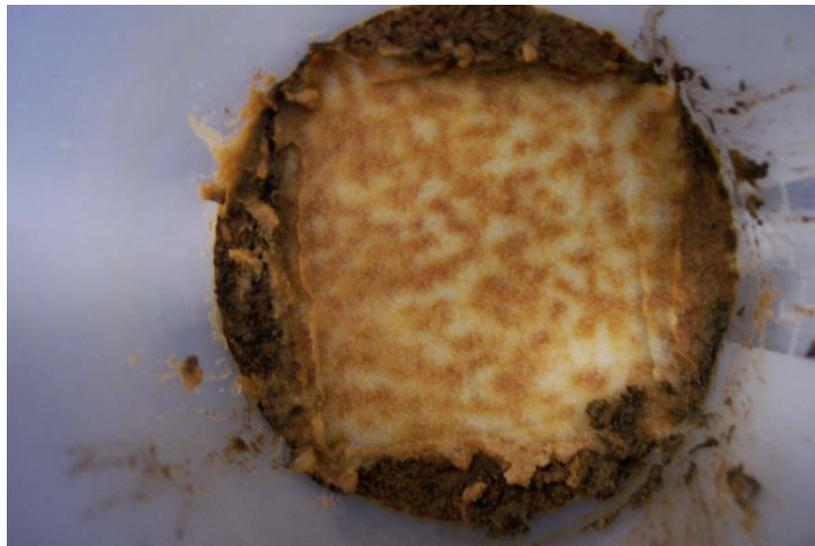
**Figure B.5** Uneven ripening of sand below the iron filings – 2
