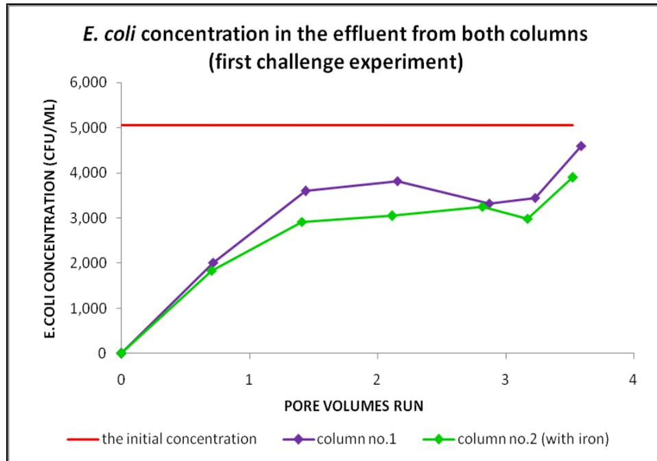
**Figure 4.4** *E. coli* removal in both columns on the 2<sup>nd</sup> day of filters operation (preliminary experiment)
