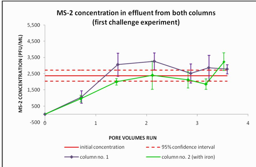
**Figure B.2 MS-2 removal in both columns on the 2<sup>nd</sup> day of filters operation (preliminary experiment – samples analyzed one day after the experiment)**
