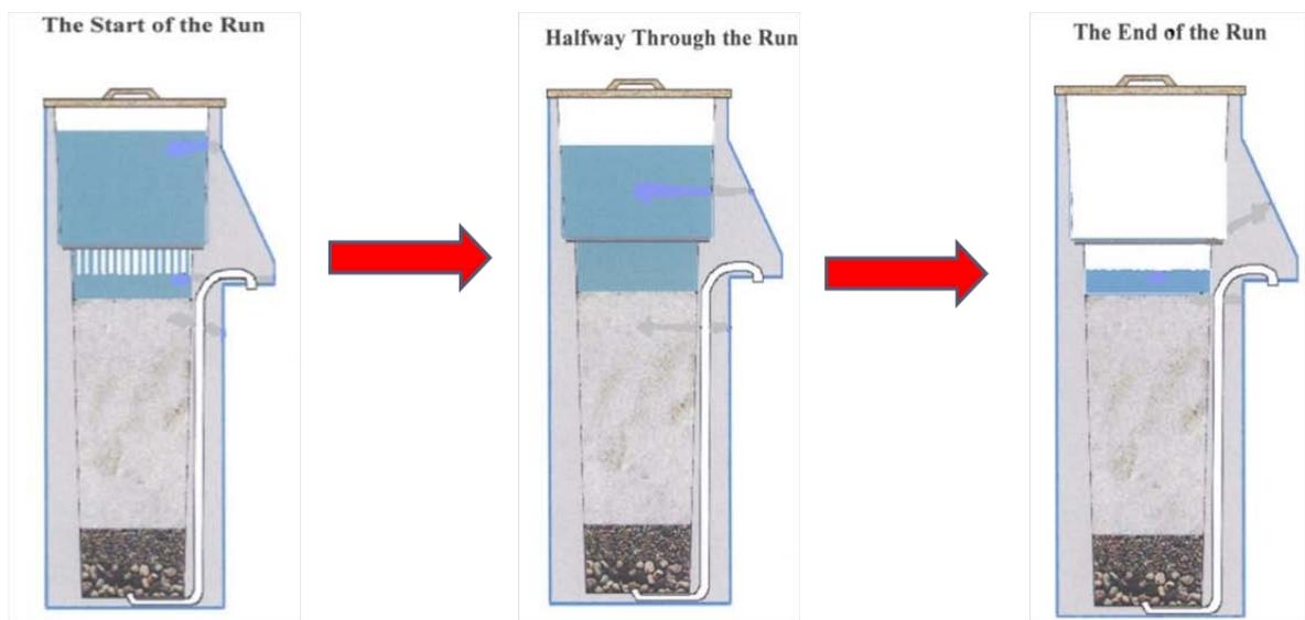
**Figure 2.1 The Biosand filter operation (Adapted from CAWST, 2008)**
