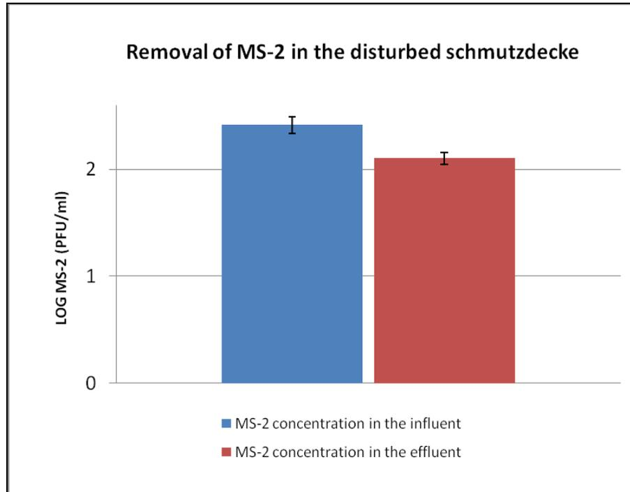
**Figure 3.13 Removal of MS-2 in the disturbed schmutzdecke**
