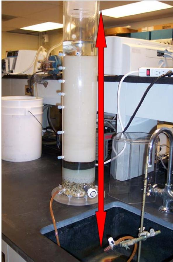
**Figure B.8 Pressure head in the second challenge experiment**
