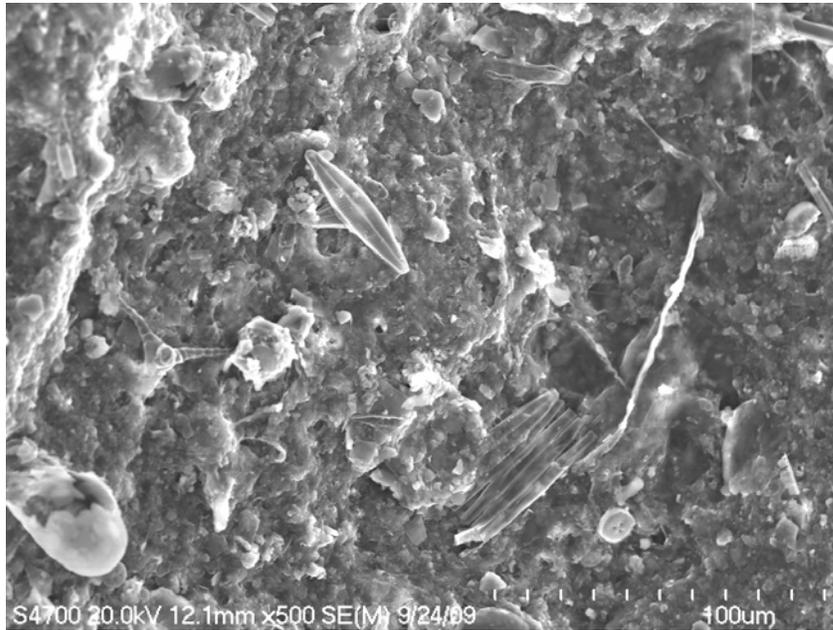
**Figure A.8 SEM picture of the schmutzdecke material (1)**
