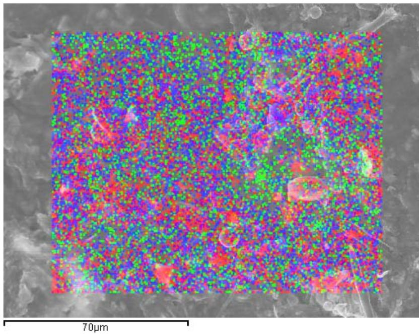
**Figure 3.14** Distribution of silica, iron, and aluminum in the schmutzdecke material (sample no. 2); Si – red, Al – blue, Fe - green
