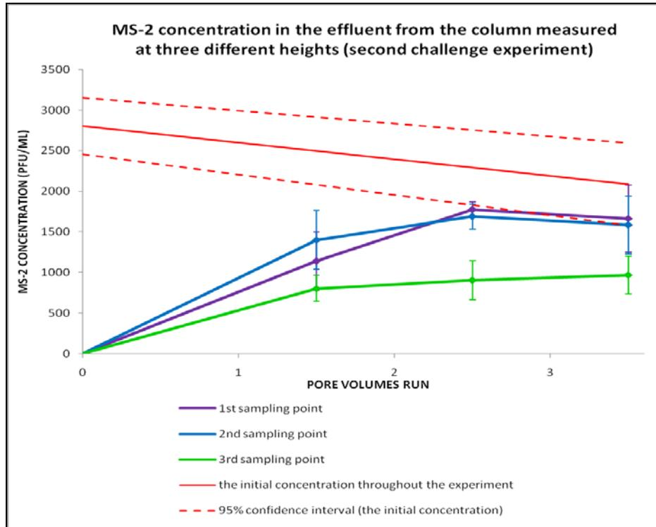
**Figure 4.11 MS-2 removal by the schmutzdecke, by the sand underneath the schmutzdecke, and by the ZVI layer on the 19<sup>th</sup> day of filters operation**
