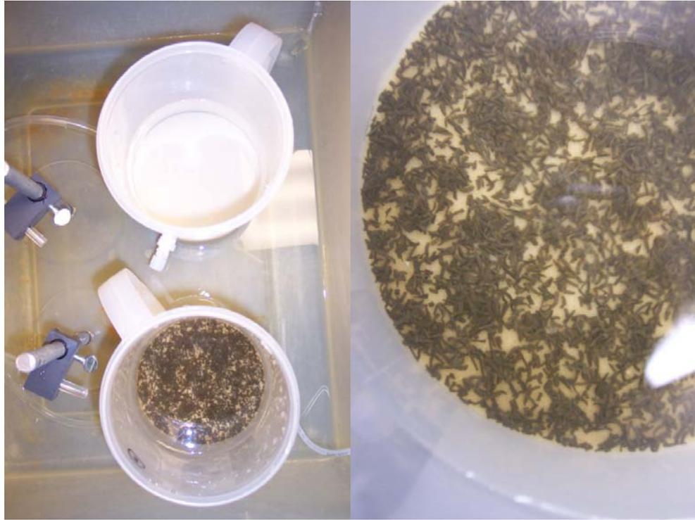
**Figure 4.1** Uneven distribution of iron over the surface of sand
