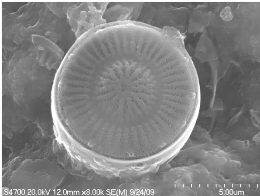
**Figure A.9 SEM picture of the schmutzdecke material (2)**
