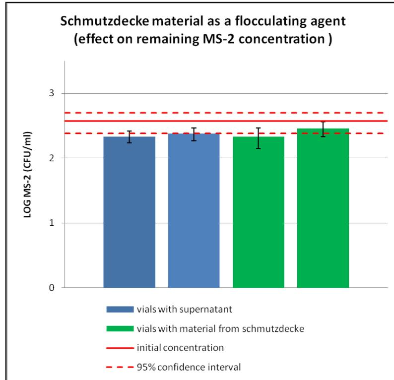
**Figure 3.16 The schmutzdecke material as a flocculating agent (effect on MS-2 concentration)**
