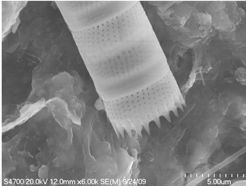
**Figure A.12 SEM picture of the schmutzdecke material (5)**
