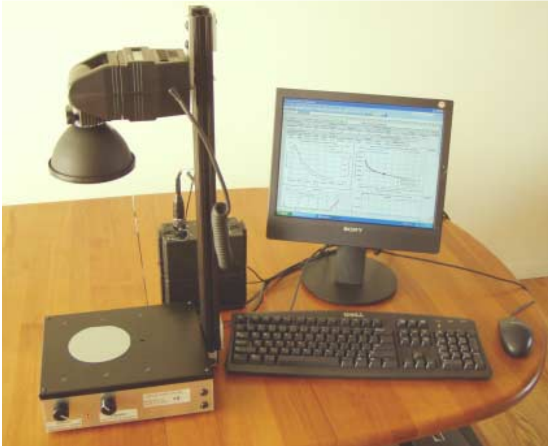
Figure 3.21 The completed system should look like this. The calibration wafer covers the sensor coil but cannot cover the small blue light sensor (standard solar cell).
