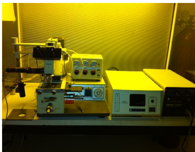
Figure 3.4 Karl Suss MJB standard 3 mask aligner used at IEC.
