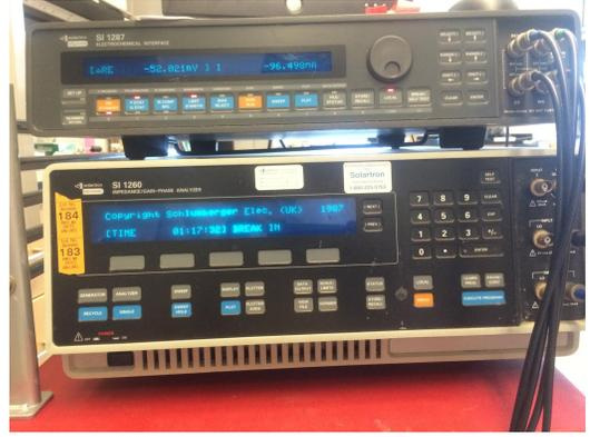
(b) Solartron Instruments 1260 and 1287
