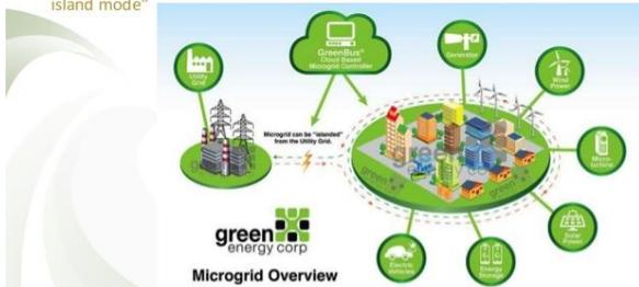
interconnections to the main grid and to most effectively balance power within the microgrid (Galligan, 2016). Microgrids can be created so that their information and distribution systems best match the energy sources and demands for the area (Galvinpower, nd).
