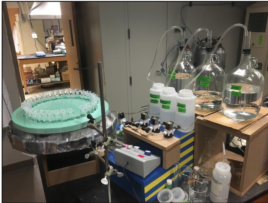
Figure 2-2. Front view of reversible sorption flow experimental setup.
