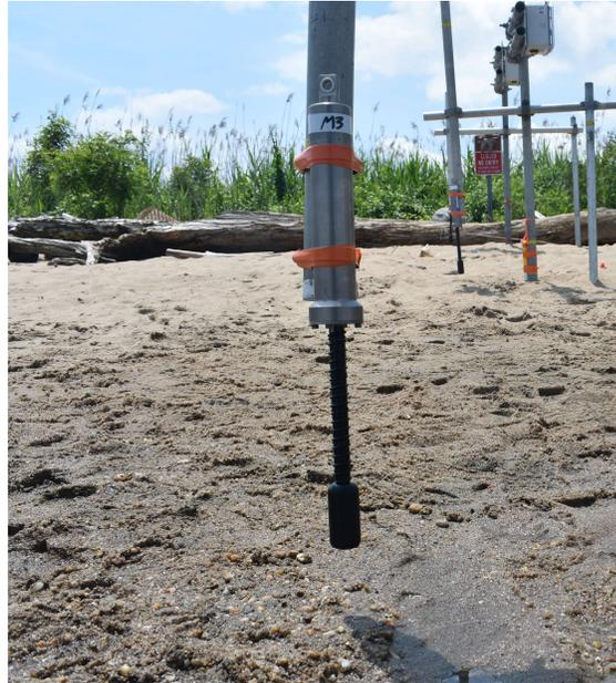
Figure 6 JFE at station M3 positioned 0.1 m above the bed. The JFEs at stations M4 and M5 can be seen in the background.
