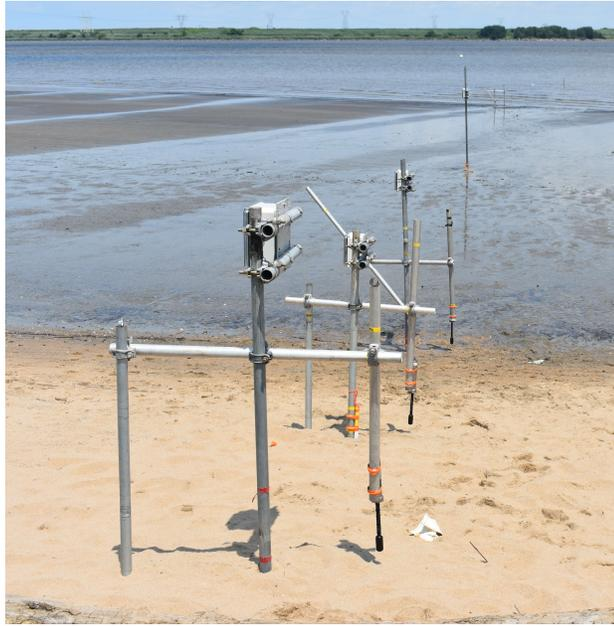
Figure 5 Stations M1-M5 set up along the transect. Stations M3, M4, and M5 are stabilized by an additional vertical pipe on the left side of the transect. Station M0 is not visible in the figure because it was submerged at the time this picture was taken.
