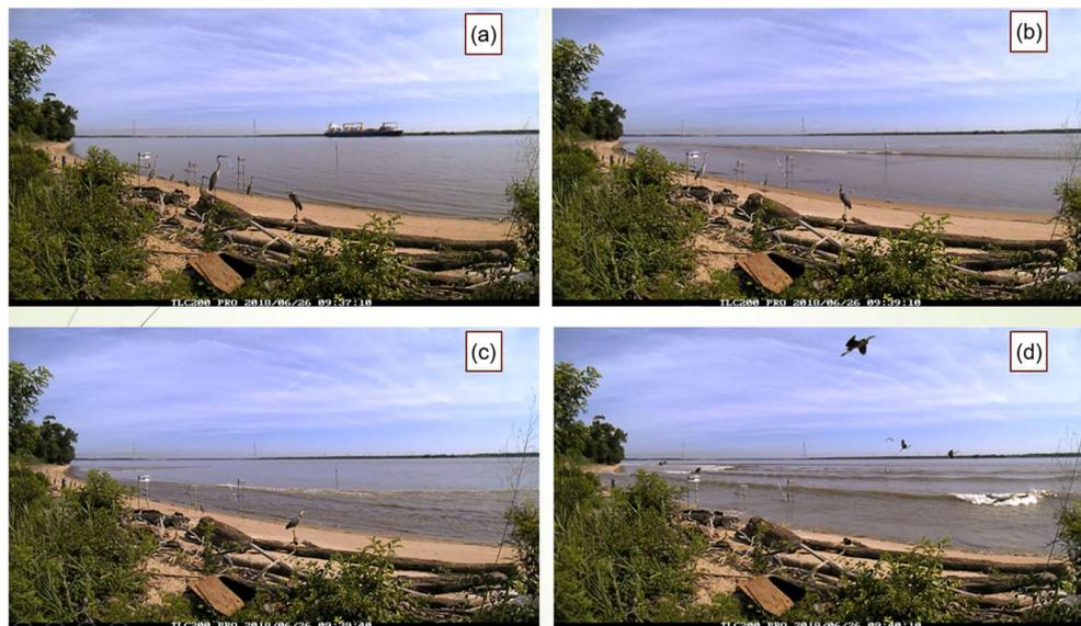
Figure 11 Time lapse imagery captured June 26, 2018. **(a)** Ship travelling south approaches study site at 9:37:10 am, **(b)** drawdown transitioning to incoming surge at 9:39:10 am, **(c)** maximum shoreward extent of surge runup has been met and remaining wave energy is reflected offshore at 9:39:40 am, **(d)** higher frequency divergent wake train propagates towards shore at 9:40:10 am.
