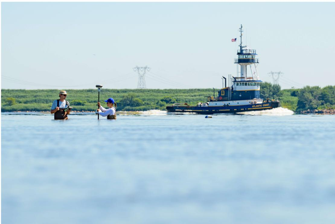
Figure 10 GNSS RTK GSP surveying along the submerged region of the transect. The orientation of this picture is looking towards the main channel from the dry beach along the study site transect. *(Picture taken by Evan Krape).*
