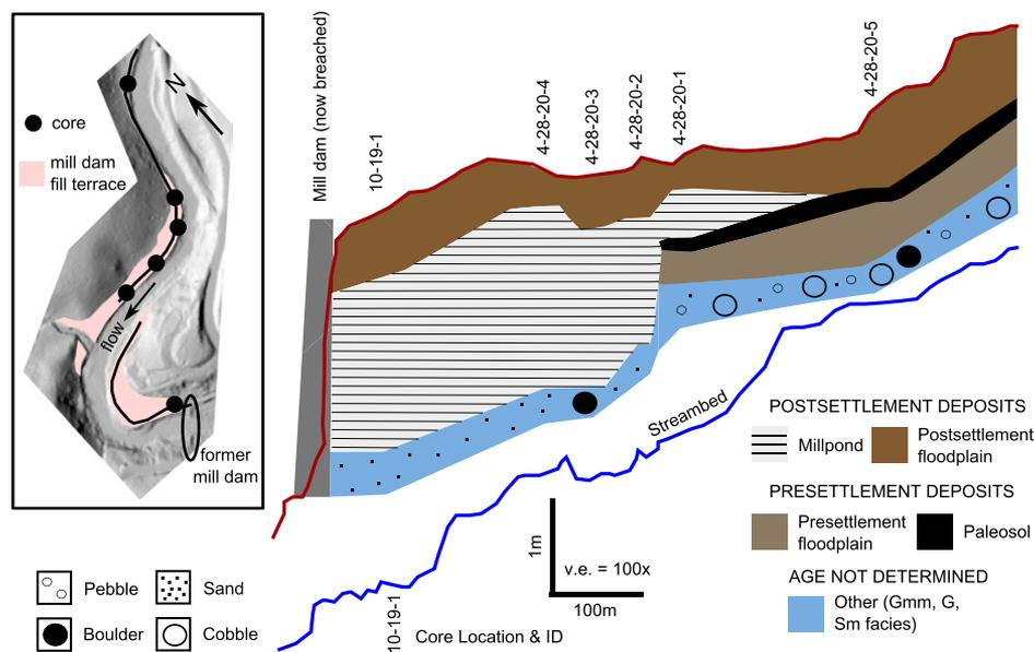
**Figure 10.** Longitudinal section at Site 6 upstream of the location of a former mill dam along the East Branch of the White Clay Creek in Pennsylvania (Fig. 1). Hillshade indicates the locations of cores, cross section, site of the former mill dam, and spatial extent of the fill terrace created by deposition upstream of the mill dam. v.e.—vertical exaggeration; Gmm—matrix-supported gravel; G—gravel; Sm—massive sand.
