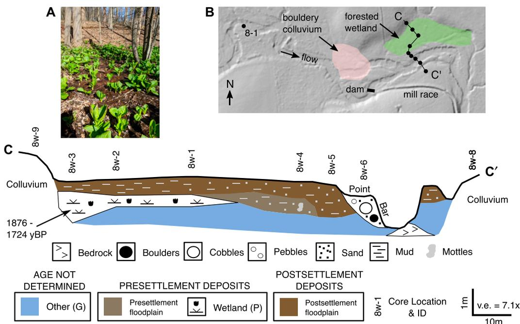
**Figure 4.** Cross section just downstream of Site 8-1 on the Middle Branch of the White Clay Creek in Pennsylvania (Fig. 1). (A) Photo showing forested wetland at location of core 8w-3. (B) Hillshade showing the locations of the cross section, an extant low run-of-river dam, coring Site 8-1, an inferred “apron” of bouldery colluvium extending across approximately half of the valley, and the extent of a forested wetland. G—gravel; P—peat; v.e.—vertical exaggeration.
