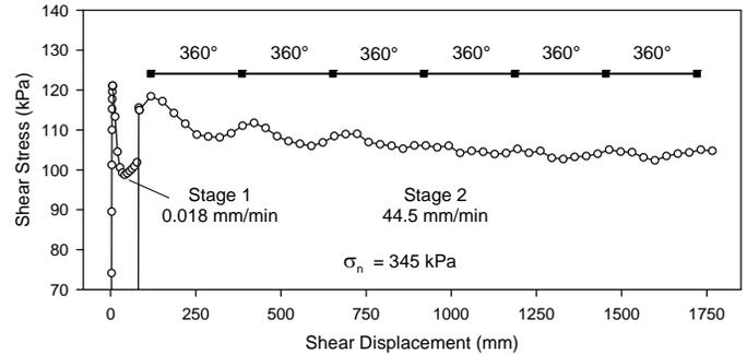
**Fig. 4:** The fast shear response of Rancho Solano Fat Clay sheared to large displacements in the Bromhead ring shear device.
