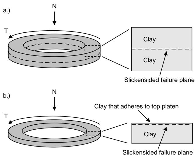
**Fig. 1:** Location of slickensided failure plane: (a) in the NGI-type ring shear, and (b) in the Bromhead ring shear.
