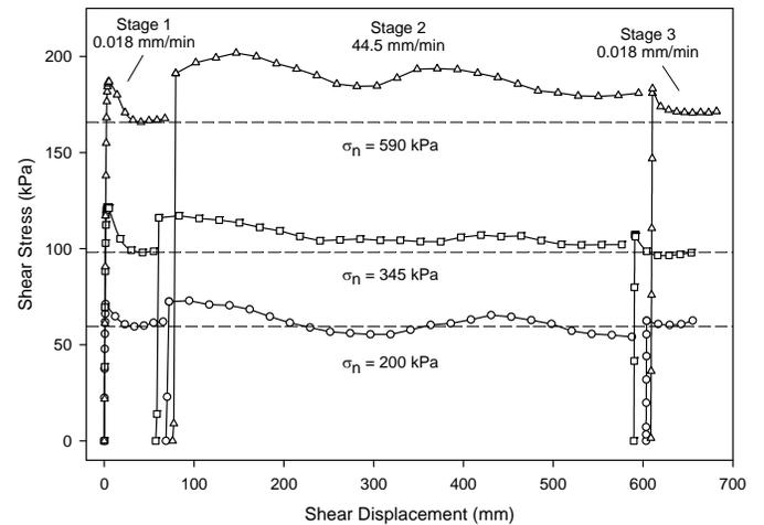
**Fig. 3:** The fast shear response of Rancho Solano Fat Clay.
