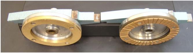
**Fig. 2:** Angle view that shows the difference between the original porous bronze platen (on the left) and the modified porous bronze platen (on the right).
