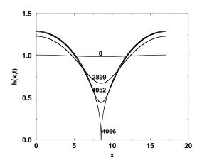
FIGURE 14. Film thickness versus spatial position for several values of time, with the Marangoni effect and no surface viscosity ( $M=1,\,\Gamma_{\rm ave}=0.75,\,{\rm Ca}=1.7,\,S=0,\,{\rm Pe}=100$ ).
