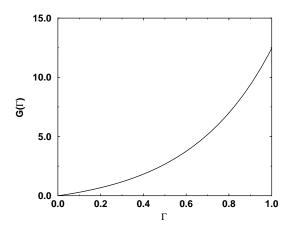
FIGURE 23. Nonlinear correlation of the surface viscosity as a function of the surfactant concentration ( $\alpha_2=2.6, (\kappa^s+\mu^s)_m=1.27\times 10^{-3} \text{ g/s [Lopez \& Hirsa (2000)]}).$
