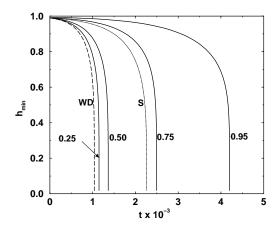
FIGURE 24. Minimum film thickness versus time for several values of the average surfactant concentration  $\Gamma_{\rm ave}$ , for variable surface properties and with the Marangoni effect (M=0.4, Ca = 1.5, S=1.27, Pe = 100). Here, curve WD denotes the Williams & Davis (1982) result (M=S=0,  $\Gamma=0$ , Ca = 1.5). Curve S denotes a result for constant surface viscosity in the absence of the Marangoni effect (M=0,  $\Gamma=1$ , Ca = 1.5, S=20).
