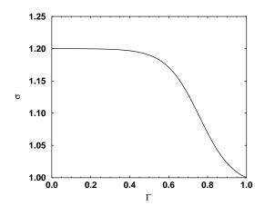
FIGURE 9. Nonlinear correlation of the surface tension as a function of the surfactant concentration, for hemicyanine in water ( $\alpha_1 = -4.4$ ,  $\bar{\Gamma}_m = 1.013718$  mg/m<sup>2</sup>,  $\bar{\Gamma}_r = 0.77$  mg/m<sup>2</sup>,  $\beta = 6.4$  dynes/cm,  $\bar{\sigma}_r = 65.9$  dynes/cm,  $\bar{\sigma}_m = \bar{\sigma}_r + \beta \tanh[\alpha_1(\gamma - 1)]$  [Vogel & Hirsa (2001)]).
