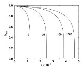
Figure 8. Minimum film thickness versus time for several values of the Boussinesq number S, for constant surface viscosity and no Marangoni effect  $(M=0,\,\Gamma=1,\,\mathrm{Ca}=1.3)$ .
