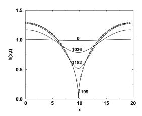
FIGURE 5. Film thickness versus spatial position for several values of time, in the absence of the Marangoni effect and surface viscosity (M=S=0,  $\Gamma=0$ ,  $\Gamma=0$ ,  $\Gamma=0$ ). The final state is the Williams & Davis (1982) result, depicted by the set with the circles.
