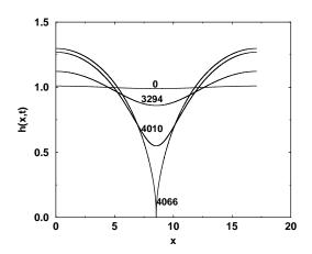
FIGURE 11. Film thickness versus spatial position for several values of time, for variable surface viscosity and with the Marangoni effect ( $M=1,~\Gamma_{\rm ave}=0.75,~{\rm Ca}=1.7,~S=1.27,~{\rm Pe}=100$ ).
