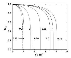
FIGURE 20. Minimum film thickness versus time for several values of the average surfactant concentration  $\Gamma_{\rm ave}$ , for variable surface properties and with the Marangoni effect (M=1, Ca = 1.7, S=1.27, Pe = 100). Here, curve WD denotes the Williams & Davis (1982) result  $(M=S=0, \Gamma=0, {\rm Ca}=1.7)$ . Curve S denotes a result for constant surface viscosity in the absence of the Marangoni effect  $(M=0, \Gamma=1, {\rm Ca}=1.7, S=10)$ .
