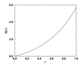
Figure 10. Nonlinear correlation of the surface viscosity as a function of the surfactant concentration, for hemicyanine in water ( $\alpha_2 = 1.9$  [Miraghaie & Hirsa (2001)]).
