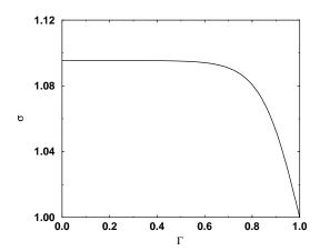
FIGURE 22. Nonlinear correlation of the surface tension as a function of the surfactant concentration,  $\sigma = 1 + (\beta/\bar{\sigma}_m) \tanh \left[\alpha_1(\Gamma - 1)\right]$  ( $\alpha_1 = -6.2$ ,  $\beta = 6.4$  dynes/cm,  $\bar{\sigma}_m = 66.2$  dynes/cm [Lopez & Hirsa (2000)]).
