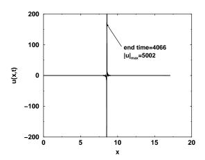
FIGURE 15. Surface velocity versus spatial position for several values of time (M=1,  $\Gamma_{\rm ave}=0.75$ , Ca = 1.7, S=0, Pe = 100). The computation terminated at t=4066 with  $|u|_{\rm max}=5002$  (not shown).
