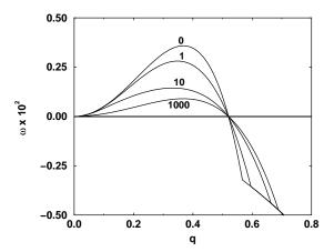
FIGURE 2. Growth rate versus wavenumber for several values of the Boussinesq number S, for variable surface viscosity and no Marangoni effect (M=0,  $\Gamma_{\rm ave}=0.75$ , Ca = 1.7, Pe = 100,  $h_0=1$ ).
