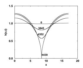
FIGURE 17. Film thickness versus spatial position for several values of time, for variable surface viscosity and with the Marangoni effect ( $M=3700,\,\Gamma_{\rm ave}=0.75,\,{\rm Ca}=1.7,\,S=1.27,\,{\rm Pe}=100$ ).
