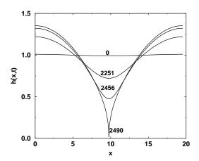
Figure 6. Film thickness versus spatial position for several values of time, for constant surface viscosity and no Marangoni effect  $(M=0,\,\Gamma=1,\,\mathrm{Ca}=1.3,\,S=20).$
