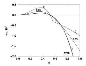
Figure 4. Growth rate versus wavenumber for several values of the Marangoni number M, in the absence of surface viscosity (S=0,  $\Gamma_{\rm ave}=0.75$ ,  ${\rm Ca}=1.7$ ,  ${\rm Pe}=100$ ,  $h_0=1$ ).
