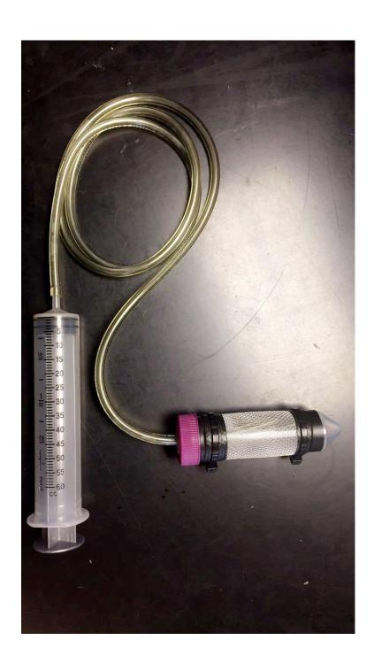
Figure 18 Ventilation design of enteric fermentation chamber to measure gas concentrations.
