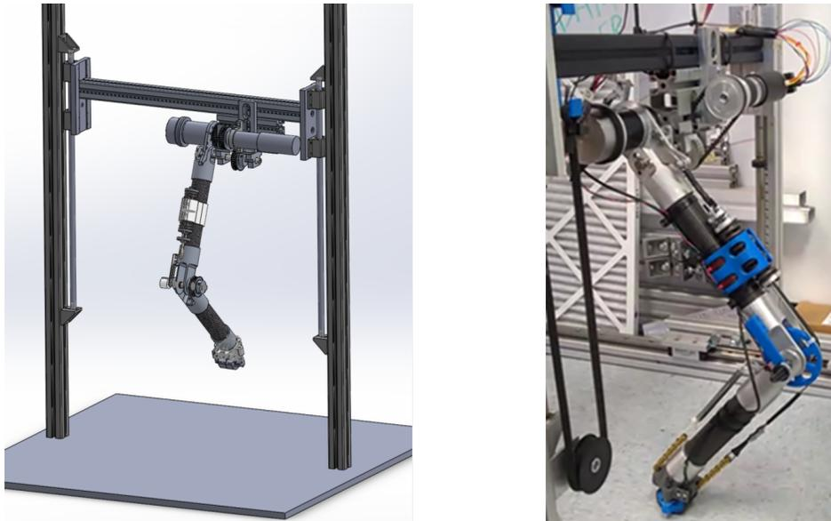
**Figure 2.6:** Left: 3D CAD Model Rendering of the SPEAR-II design with slider boom. Right: Photo of SPEAR-II robot in stance phase.
