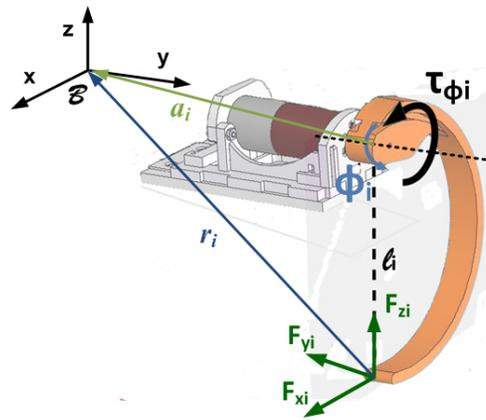
Figure 2: Modeling of Leg Forces (Reproduced from [7] with permission)
