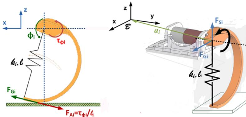
Figure 3: Leg Forces on the  $(x-z)^B$  plane (Reproduced from [7] with permission)
