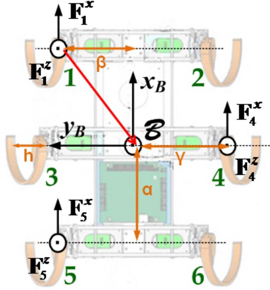
Figure 4: Allocation of Leg Forces (Reproduced from [7] with permission)
