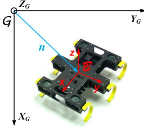
Figure 1: Global  $G$  and Body-fixed  $B$  Coordinate Frames (Reproduced from [4])
