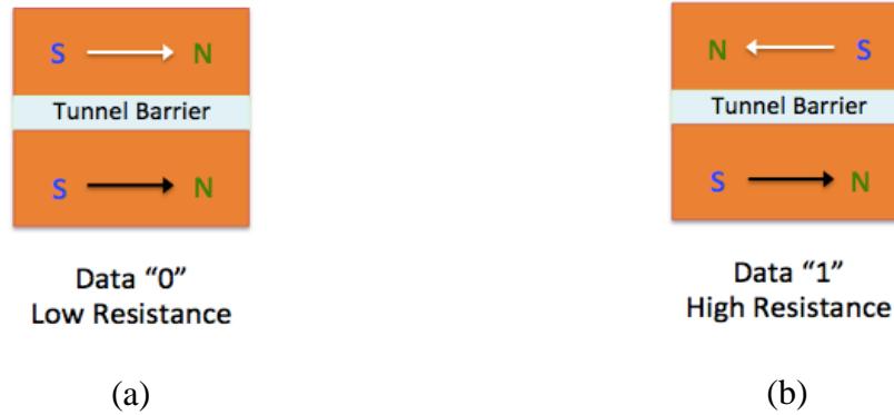
Figure 4.1 Simplified schematic of magnetic tunnel junction element at two distinct resistance states.
